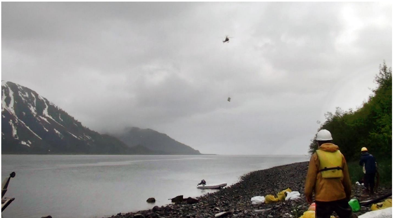
Sling loads of nets and other debris transferred to Macleod Harbor from Point Bryant. The nets were cut into large chunks and loaded into Super Sacks for helicopter slinging.
